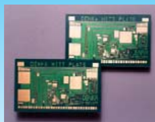
DENKA HITT PLATE (Al-base substrate/IMS)
