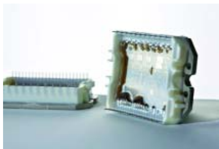
Figure 1 and 2: Using UV-active silicone gel from WACKER SILICONES to encapsulate an electronic component.
