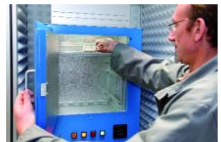
Figure 4: With the aid of a special UV-exposure chamber, WACKER engineers in Burghausen can test the novel UV silicone gels' properties, such as rapid curing and variable control of curing times.
