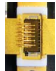
Figure 4: At left are the pulsed output characteristics at V gs = 3 V for 1200 V normally-off SiC JFET showing a room-temperature saturation current over 100 A. At right is a picture of the 15 mm 2 normally-off SiC JFET assembled in Kyocera A0883 LD MOS package. Package was selected strictly for the purpose of device characterization and is not representative of the product packaging [A. Ritenour et al.].
