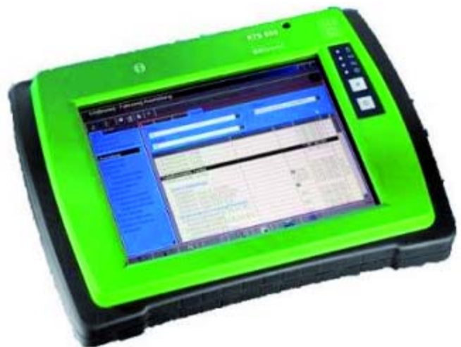
Figure 2: With the help of Kontron MARS, mobile applications — such as the diagnostic system for automobiles shown here — can be supplied with uninterrupted energy: A fall back battery allows to replace the discharged battery without intermission.
