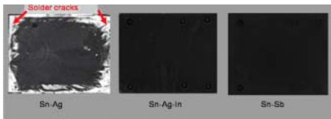
Figure 5: Comparison of crack areas between Sn-Ag solder, Sn-Ag-In-solder and Sn-Sb solder between Si 3 N 4 -DCB and copper base plate after 300 thermal cycles.
