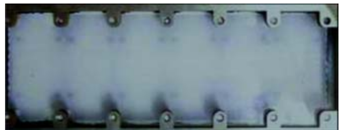
Figure 7: spreading behavior after tighten up the screws
