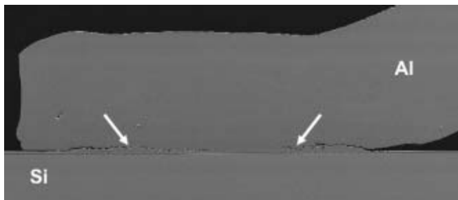
Figure 1: Cross section of a bond showing cracks growing from either end of the wire towards the center of the bond
