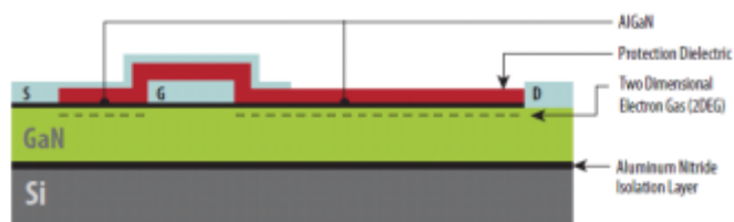
Figure 1: GaN on silicon devices have a very simple structure similar to a lateral DMOS device and can be built in a standard CMOS foundry
