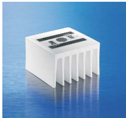
Figure 4: First serial production of optimized CeramCool geometry for 4W cooling. With Rubalit the total thermal resistance R_{th} of the assembly is at least 13% better than aluminum. Using Alunit it is more than 31% better.
