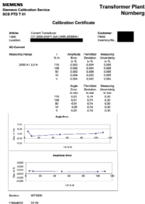
Figure 5: Calibration protocol of a 2000 A transducer. Even at low range of 50 A the accuracy is better than 0.005 % and the phase error below 0.05 min
