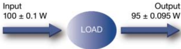
Figure 4: Deviations of input- and output power measured with a power system of 0.1 % accuracy
