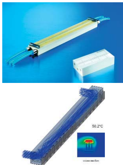
Figure 6: CeramCool liquid cooling allows almost any needed cooling capacity. With Rubalit ceramics the power density of 290W is managed with only 120mm lengths. The cooling water is only 1.5mm away from the LED heat slug. The solution is now available from extruded Alunit – a breakthrough in production engineering. While Rubalit dissipates 290W on 120mm, Alunit can cool 640W!
