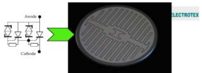
Figure 5: Experimental dinistor semiconductor element
