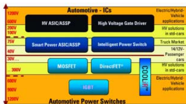
Figure 1: IR's Automotive Product portfolio of AEC-Q100 qualified Power switches and AEC-Q101 qualified ICs and their typical applications fields in cars trucks and (hybrid) electric vehicles
