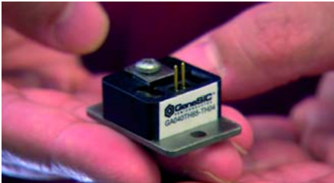
Figure 2: GeneSiC recently introduced 6.5kV-class Silicon Carbide Thyristors to researchers investigating utility-scale power conversion circuits.
