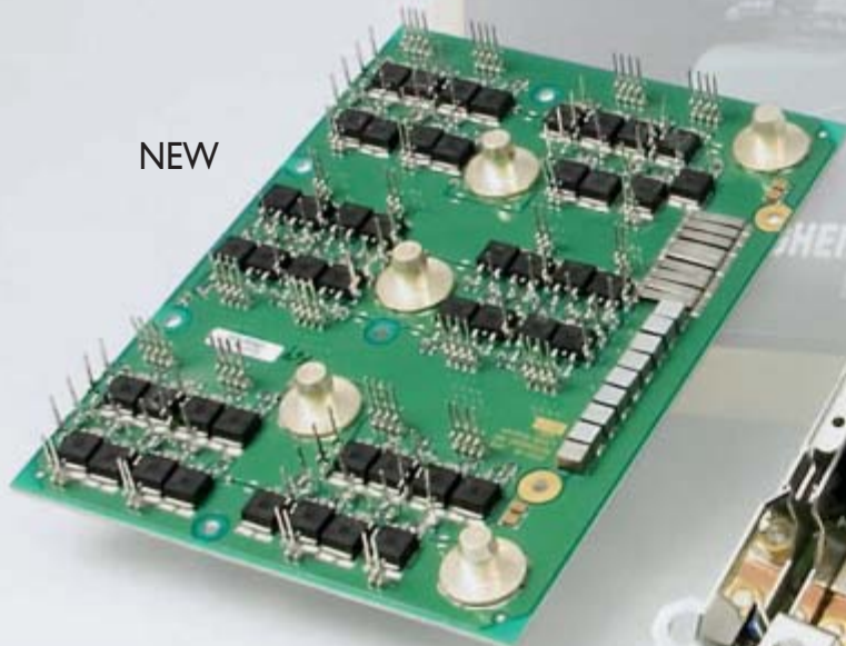
POWER BOARD ASSEMBLY (ACTUAL) (48) FETs (9) Low profile capacitors (5) Low profile bus bars TotalWt. 370.6g
