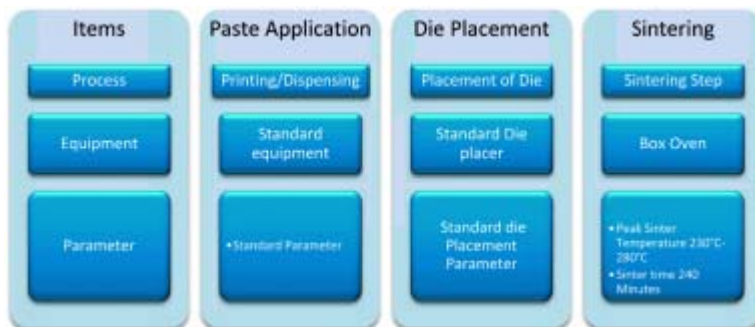
Figure 7: Example of Process flow for no pressure sintering process of mAgic 016 Paste Series with die sizes up to 100mm 2
