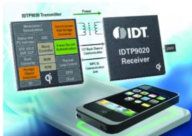
Figure 1: A wireless power charging system using IDT's IDTP9030 and IDTP9020 devices
