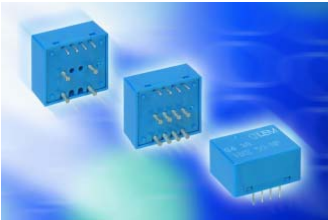
Picture 1: LEM's HXS series: Open Loop Hall effect based current transducers using the previous LEM ASIC generation
