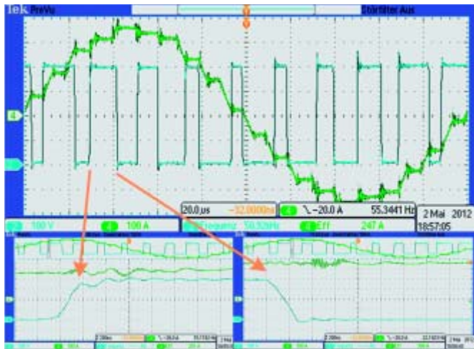
Figure 4: Load currents at 5kHz frequency (top), PWM up and down swing (bottom)
