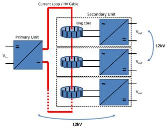
Picture 2: Block Diagram of IPSS
