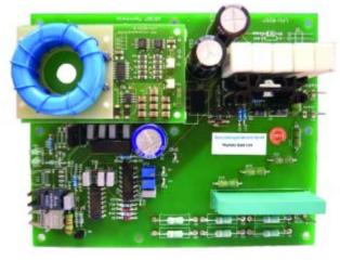
Picture 3: Thyristor trigger unit (TTU)
