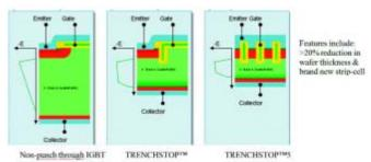
Figure 1: Infineon's IGBT technology evolution
