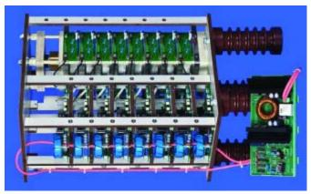
Bild 5: Thyristor Pulser Bidirectional W1C 12kV / 32kA
