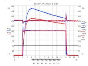
Figure 5: Trench XPT IGBT short circuit characteristic
