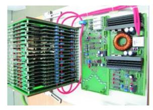
Picture 7: IGBT DC Switch, E1C 16kV /10A with IPSS, IGBT driver, senses, diagnostic, communication interface and potential free feedback.
