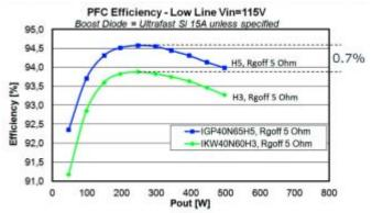
Figure 4: turn off switching comparison between H3 and H5<sup>2</sup>
