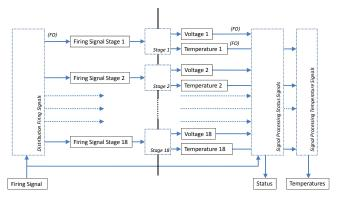
Bild 6: Block diagram of medium voltage switch W1C 24kV / 600A
