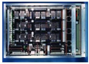
Picture 9: .....e.g. IGCT 3-Level-Inverter-Stack
