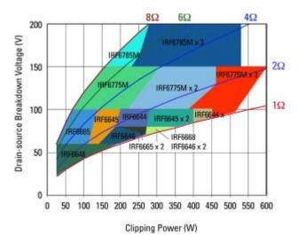
Figure 1: MOSFET selection based on voltage rating and audio output power
