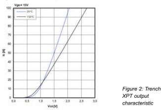
The Trench XPT has a low VCE(sat) (1.5V @lnom,25°C & 1.75V @lnom, 150°C). The positive temperature coefficient of the Trench XPT provides a negative feedback, making the XPT suitable for paralleling in modules or circuits. In addition to the low VCE(sat) the Trench XPT also has a low off-state leakage current at 150°C (<100 $\mu$ A @650V). The switching characteristics of the 50A, 650V Trench XPT are shown in figures 3 & 4.
