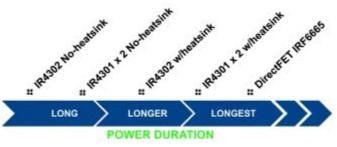
Figure 4: Amplifier architecture selection by power duration
