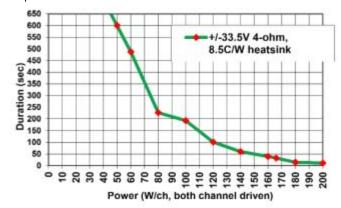
Figure 3b: Extending power duration by adding small heatsink
