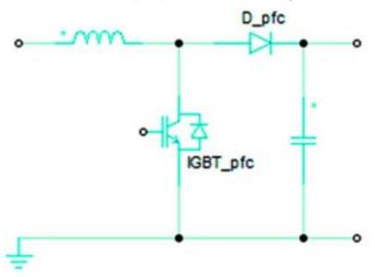
Figure 5: Standard PFC configuration used for comparison analysis
