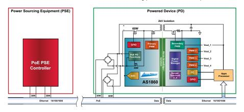
Figure 2: Interoperability of Broadcom's PoE PSE controller (BCM59111) and Akros' SoC IC (AS860)
