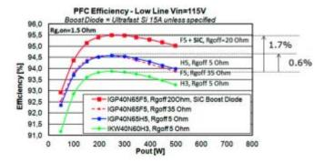
Figure 6: 70 kHz PFC measurement comparison
