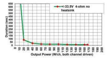
Figure 3a: Power duration for heatsink-free design using a single amplifier IC
