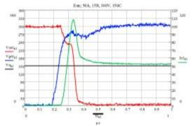
Figure 4: Trench IGBT turn-on characteristic
