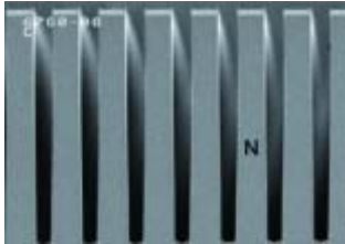
Figure 4: Cross section of the SJ deep-trench structure developed by Renesas
