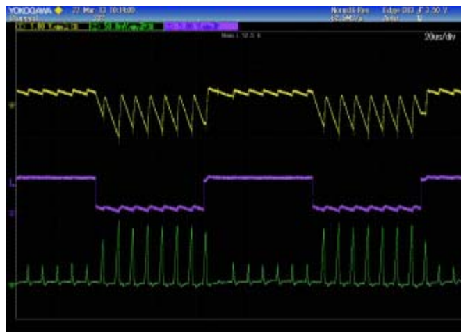
Figure 6: PEB Amplifier Running as a DC/DC Converter with a Step Load
