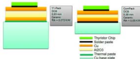
Figure 4: improved thermal construction (ComPack)
