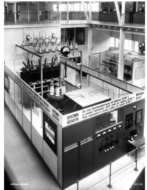
Figure 4: A simple rectifier circuit with a 6 anode mercury-arc rectifier equivalent to an H-bridge (Source: Wikipedia)
