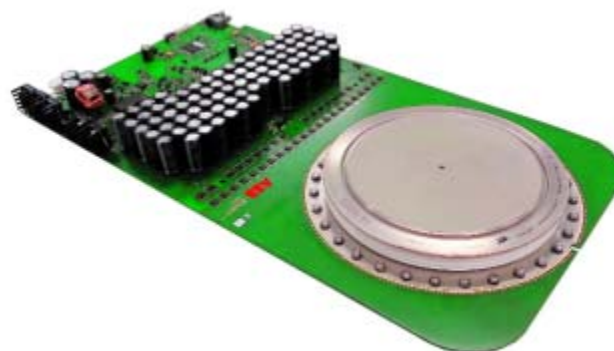
Figure 3: 150mm 4,500 V RC-IGCT (Prototype)
