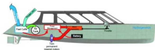
Figure 3: Schematic of the power system used in the Hydrogenesis
