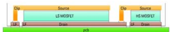
Figure 1a: Conventional two-clip dual PQFN package construction featuring individual clips connected to sync (LS = Low-Side) MOSFET and control (HS = High-Side) MOSFET, (LF=Leadframe).
