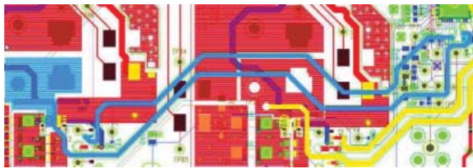
Figure 3: PGND and LX Return conductors shown in Blue on Layer 4
