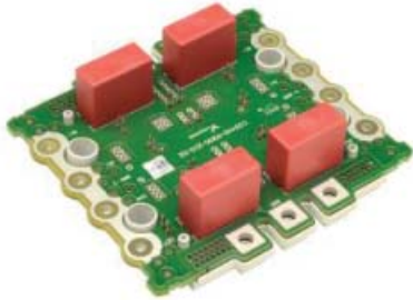
Figure 11: Power module mechanics with power connection and low inductive interface
