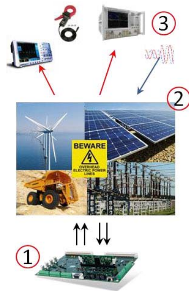
Figure 1 Power electronics test stand, the conventional way; 1 - digital controllers; 2 - high power systems; 3 - measurement and testing equipment
