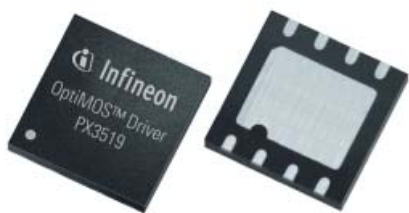
Figure 3: PX3519 VDSO-8 in leadless package
