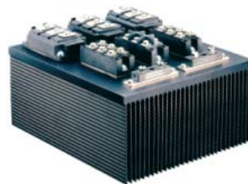
Figure 3: IGBT modules placed onto the heat sink
