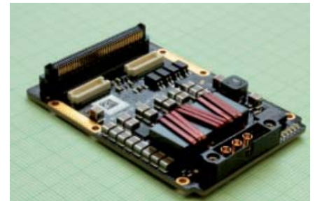
Figure 4: Topside of the Si-Inverter signal near the center is generated by driving an inductive load.
