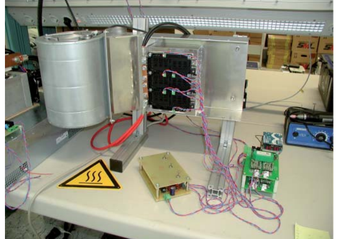
Figure 3: Test bench to evaluate thermally induced pump-out effects
