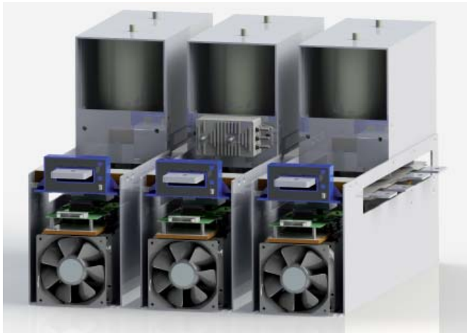
Figure 3: The link system facilitates the connection of the units into a 3-phase inverter extremely
