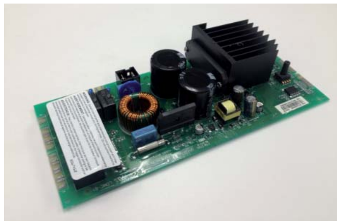
Figure 4: Appliance control board upgraded to 850W using SiP IRAM Gen2 IPM
