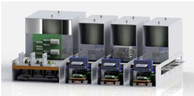
Figure 4: The appropriate VARIS™ R (left) rectifier docks easily onto the existing inverter
