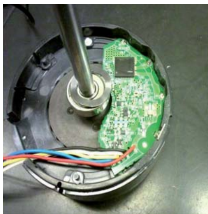
Figure 2: Designing with \mu IPM allows engineers to realise extremely compact motor drivers
