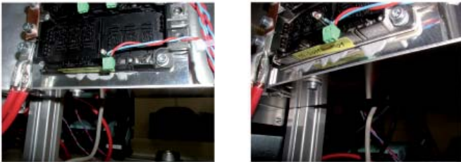
Figure 4: Left side - Stamp A after 45 cycles with massive pump-out. Right side - Stamp B after 1200 cycles with reduced pump-out effect
