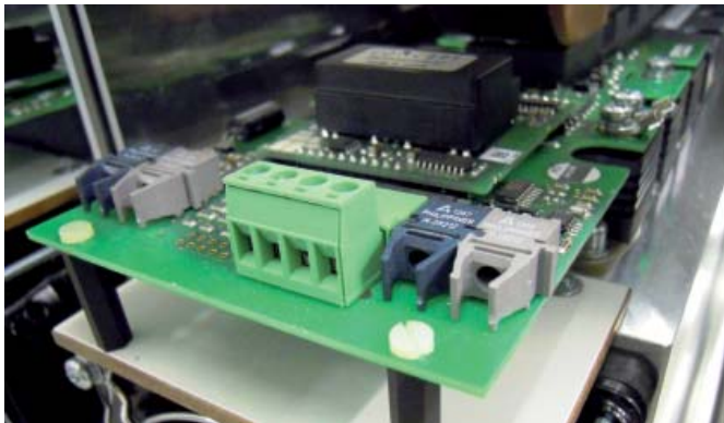
Figure 7: The plug & play driver for the PrimePACK™ modules is a development of GvA
