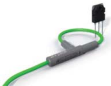
Figure 1: A CWT Mini coil, insulation voltage 2kV peak, thickness 3.5mm, coil length 100mm, threaded through the legs of a TO-247 semi-conductor package.
