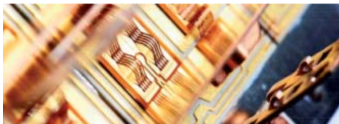
Figure 1: A protective layer of copper was added to the chip allowing the use of superior copper wires
