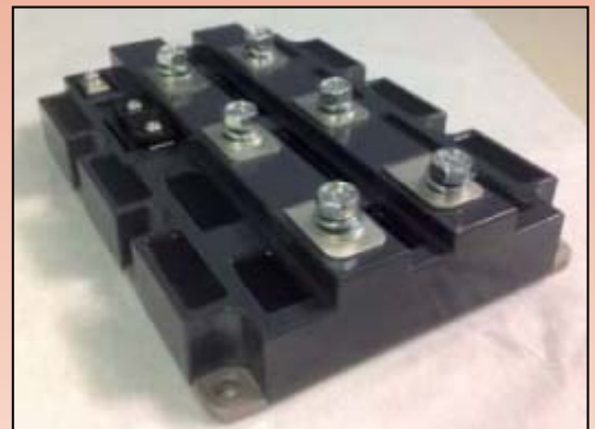
CCS-MD-20N33A70, 2000A, 3.3kV, single switch
