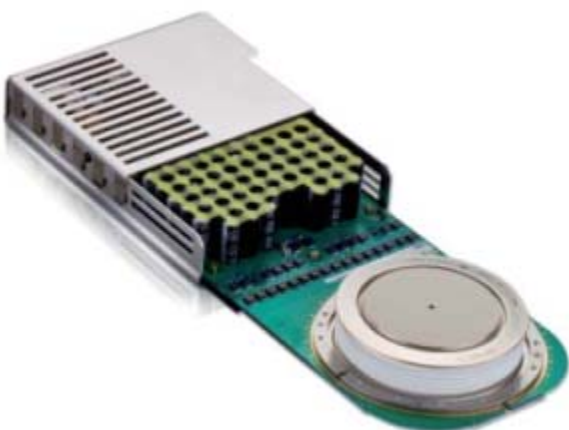
Figure 3: Asymmetric 4.5 kV IGCT, the device of choice for demanding high-power applications.
