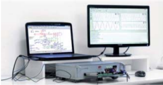
Figure 3: Full design, simulation, prototyping, testing, and verification of the controller is done from the comfort of the engineer's desk. Grid-connected inverter is running in real-time in HIL configuration, controlled with automatically generated code from PSIM.
