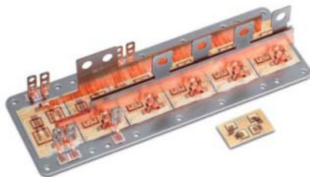
Figure 2: Due to the improved vertical current flow, there is no longer a need to place a stitch bond on the semiconductor
