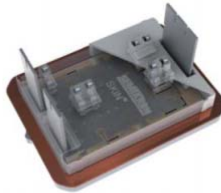
Figure 4: 3D SKiN® module comprising of 6 x IGBTs and 6 x FWDs
