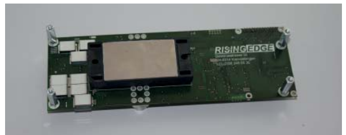
Figure 6: The unpopulated motor control: The first step is the assembly of the output stage, an integrated three-phase full-bridge module with six MOSFETs. Caption: Rising-edge
