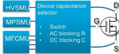
Figure 20: Agilent B1507A Hardware Block Diagram
