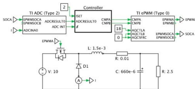
Figure 4: Current-controlled buck converter with peripheral models
