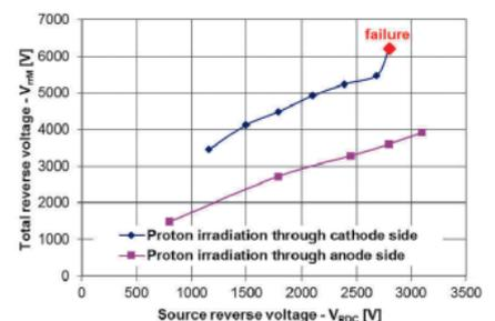
Figure 8: Dependencies of the total reverse voltage ( $V_{\text{rrm}}$ ) on power supply reverse voltage ( $V_{\text{RDC}}$ ) for the diodes produced using the conventional technology and for the experimental diodes.
