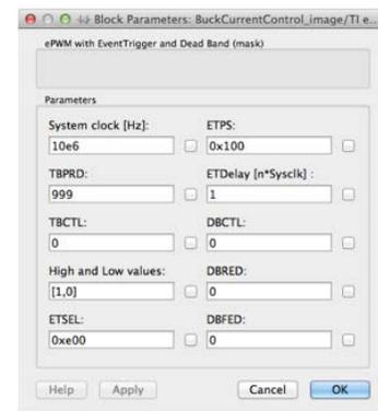
Figure 3: Model of a TI Type 0 ePWM module implemented in PLECS
