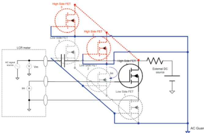
Figure 13: 6 in 1 Module, Crss measurement at High Voltage Basis
