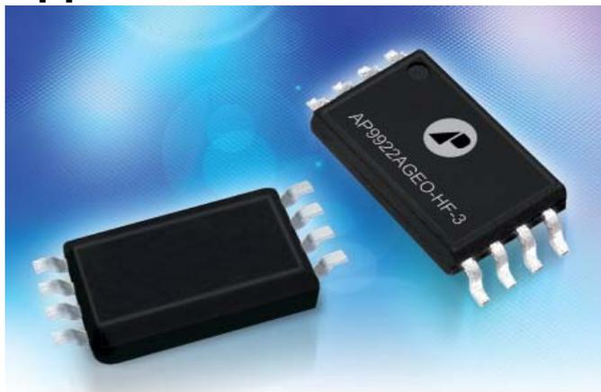
Advanced Power Electronics Corp. has announced a new dual N-channel enhancement-mode power MOSFET well-suited for battery applications. The AP9922AGEO-HF-3 device supports 1.8V gate drive and features a low on-resistance of 18mΩ, a drain-source breakdown voltage of 20V and a continuous drain current of 6A. RoHS-compliant and halogen-free, the device is available in the small and thin TSSOP-8 package.
