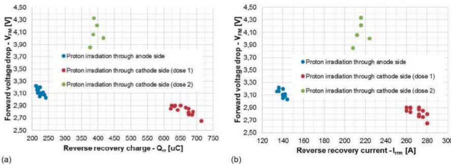
Figure 3: Correlation of  $V_{FM} / Q_{rr}$  (a) and  $V_{FM} / I_{rrm}$  (b) for the experimental diodes (proton irradiation from the anode side) comparing to the diodes produced using the conventional technology (proton irradiation from the cathode side)
