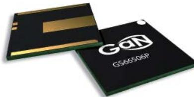
chip-scale, embedded GaNPX package which eliminates wire bonds thereby minimising inductance. This package also optimises thermal performance and is extremely compact.
