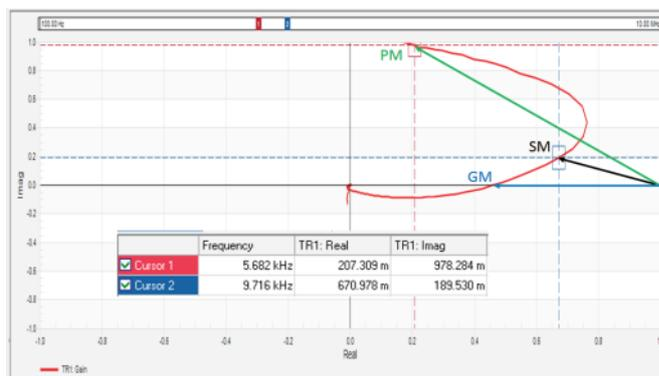
Figure 5: Nyquist chart created from the Bode plot data in Figure 2 shows the phase margin, gain margin, and stability margin.
