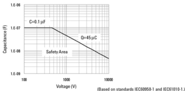
Figure 9: Capacitance Charge generally considered as safety
