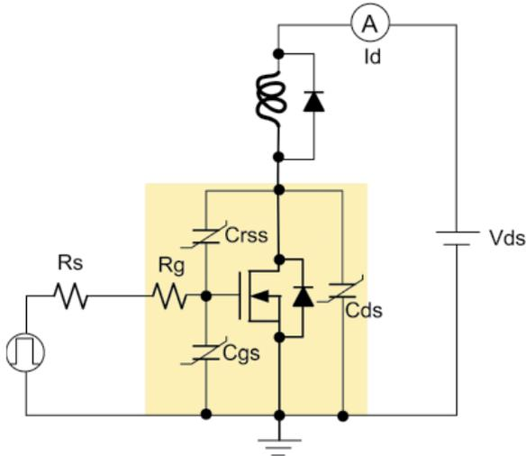
Figure 18: Apply device capacitance to simulator
