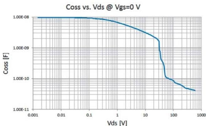
Figure 16: Coss voltage dependency
