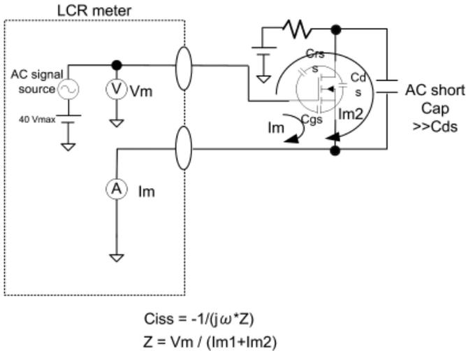
Figure 12: Crss measurement for normally on device at High Voltage Basis
