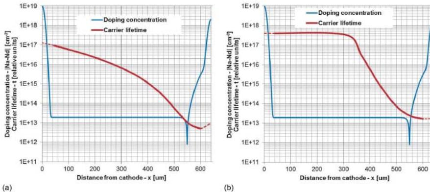
Figure 2. Typical carrier lifetime distribution (t) during proton irradiation through the cathode surface of the semiconductor element (a) and during proton irradiation through the anode surface of the semiconductor element (b)
