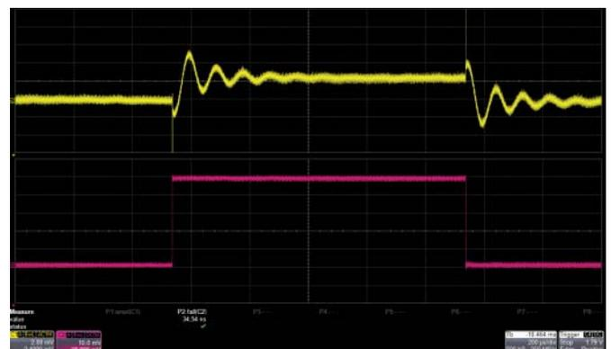
*Figure 3: 500mA Step load response of the DC/DC converter. The upper trace is the output voltage at 2mV/div. the lower trace is the current step at 100mA/div and the timescale is 200us/div. The rise and fall time of the step are 35ns.*
