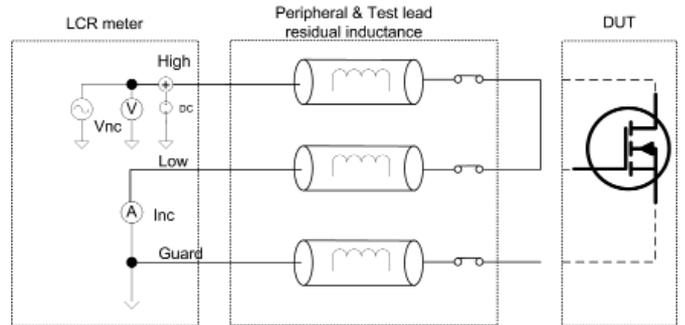
Figure 14: Short correction including Guard terminals is required for compensating residual inductance
