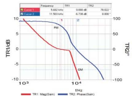
*Figure 2: Bode plot of a DC/DC converter.*
