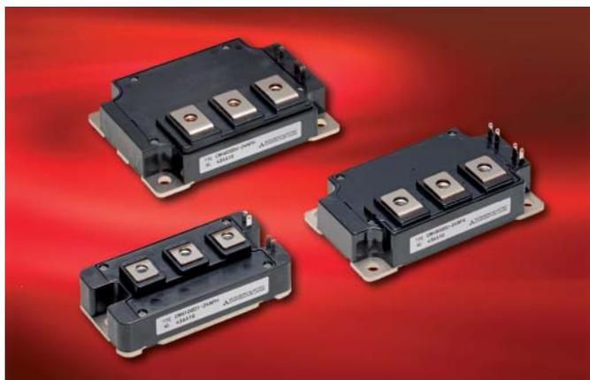
40%. Featuring SiC Schottky Barrier Diodes (SBD) and Silicon IGBTs, the modules achieve high efficiency, downsizing and weight reduction in inverters. The Modules are designed for typical switching frequencies of more than 20 kHz.
