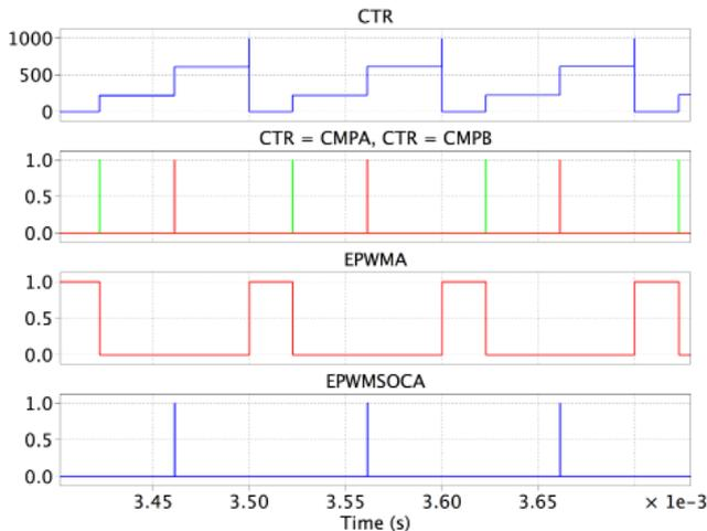
Figure 5: PWM modulation and conversion trigger based on the ePWM model
