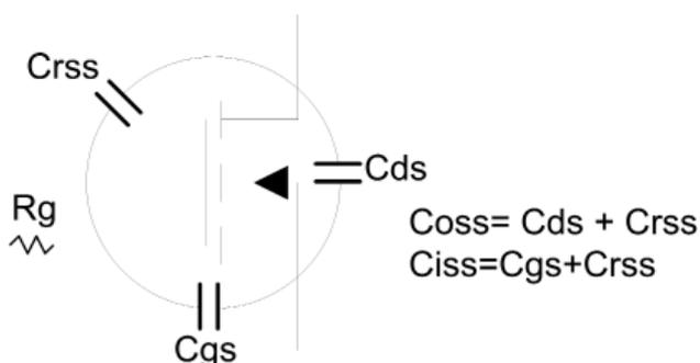
Figure 1: Three Capacitance of Power MOSFET
