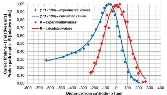
Figure 1: Typical relative carrier lifetime distribution ( $1/\tau_1 - 1/\tau_0$ ) and proton path depth  $R_p$  in semiconductor element after proton irradiation with initial energy of 24 MeV.  $\tau_1$  and  $\tau_0$  – carrier lifetime values before and after irradiation.
