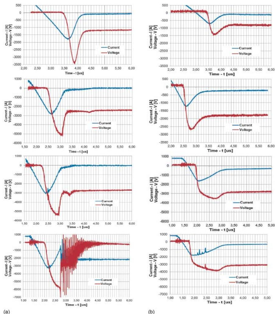
Figure 6: Oscillograph records of anode current and voltage during reverse recovery for the diodes produced using the conventional technology (a) and experimental diodes (b) at various reverse voltage values  $V_{RDC}$ .
