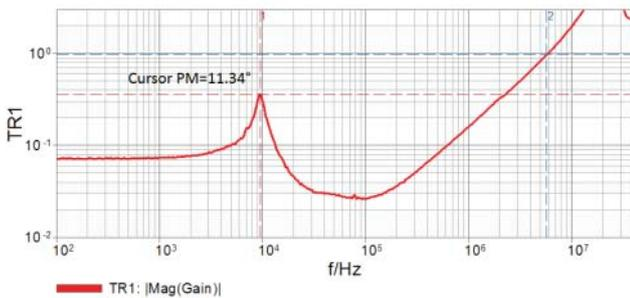
Figure 7: Output impedance measurement and cursor reported stability margin.
