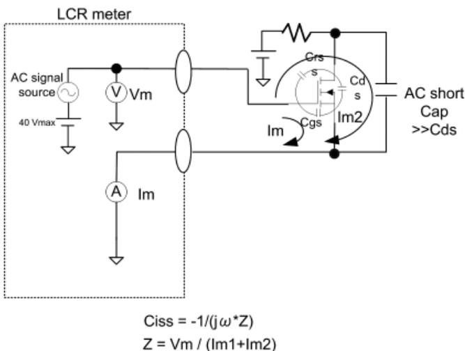
Figure 4:  $C_{iss}$  measurement by LCR meter
