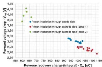
Figure 4: Correlation of  $V_{FM} / Q_{rr-i}$  for the experimental diodes (proton irradiation from the anode side) comparing to the diodes produced using the conventional technology (proton irradiation from the cathode side)
