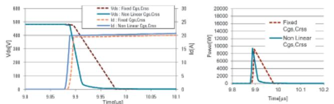
Figure 22: Simulated switching characteristics and power loss
