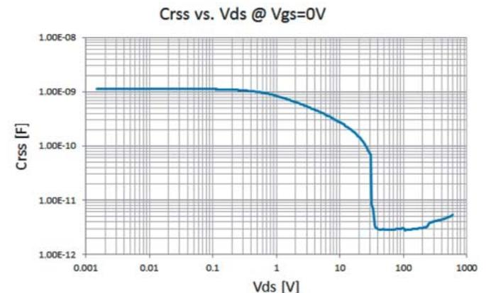
Figure 15: Crss voltage dependency
