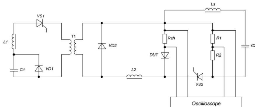
Figure 5: Circuit of experimental equipment to study the reverse recovery characteristics at high change rate of reverse recovery current ( $di_{rrm}/dt$ ) and power supply reverse voltage ( $V_R$ )
