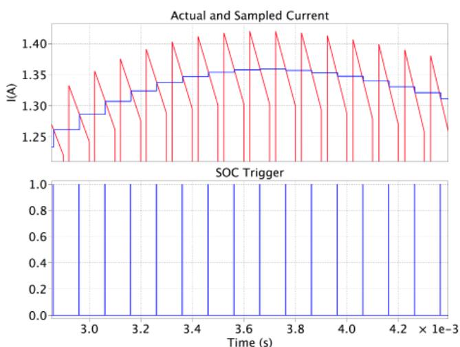
Figure 6: Current measurement invoked by the ePWM module
