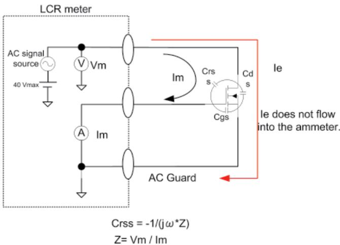
Figure 3:  $C_{rss}$  measurement by LCR meter
