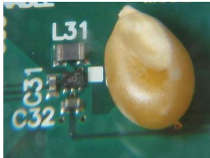
*Figure 1: A recently introduced switching regulator along with a single popcorn kernel clearly showing the limited access for injection and measurement probe for stability assessment. The POL regulator also lacks access to the feedback loop.*
