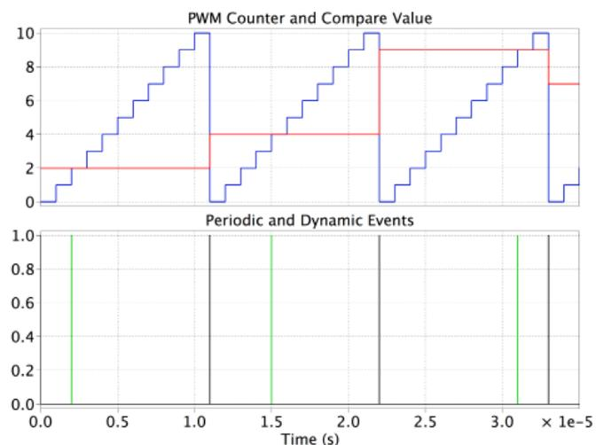
Figure 1: Typical counter behavior of a PWM module
