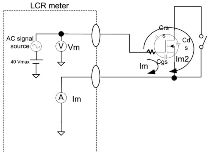
Figure 5:  $R_g / C_{iss}$  measurement by LCR meter
