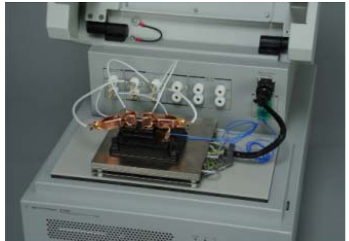
Figure 4: Thermal plate in B1506A test fixture
