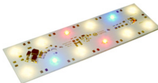
Figure 5: Customized LED module for sea life aquariums
