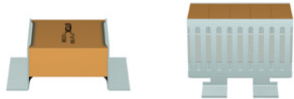
Figure 2: SMD CeraLink for integration in IGBT modules. The CeraLink low-profile 1 \mu F variant (left) and the 5 \mu F type (right) are designed for embedding in IGBT modules. They feature compact dimensions and can withstand high temperatures of up to 150 °C.
