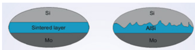
Figure 1: No partial dissolving of silicon surface layers on the anode side
