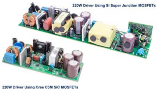
Figure 3: Side-by-side comparison of two 200W LED drivers: one using Si superjunction MOSFETs and two-stage topology, and the other using a Cree® C3M™ SiC MOSFET and single-stage topology.
