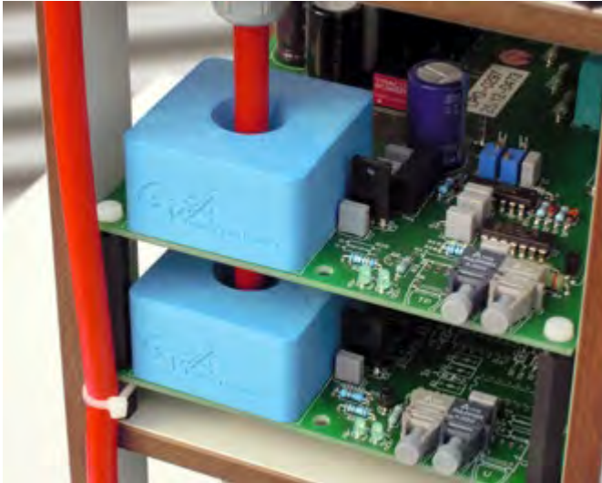
Figure 2: In the IPSS the decoupling units on the control boards ensure the inductive transmission of the required power
