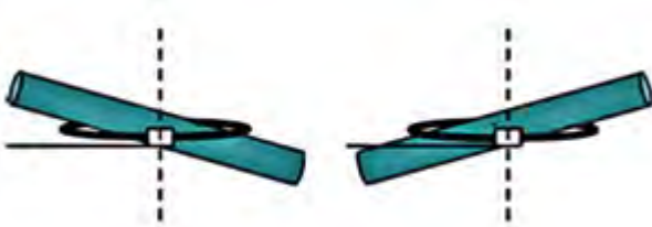
Figure 7: Orthogonality effect. Primary conductor position versus the axis of the Rogowski loop.
