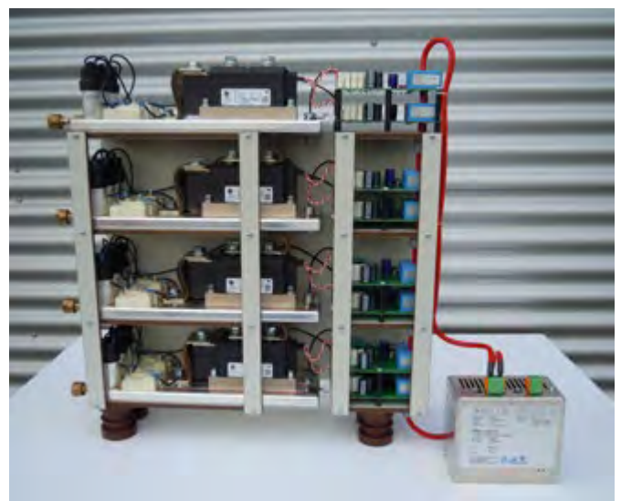
Figure 1: The auxiliary power supply units such as the 'Inductive Power Supply System (IPSS)' from GvA sensibly specify the test voltages free of partial discharge
