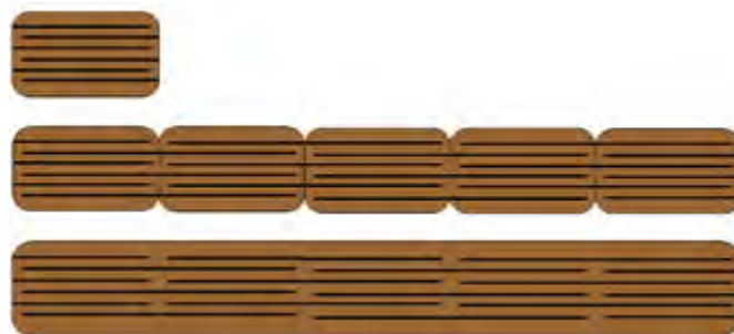
Figure 4: Top: Five individual capacitors in series. Bottom: Monolithic series-electrode construction raises the breakdown voltage but reduces capacitance.
