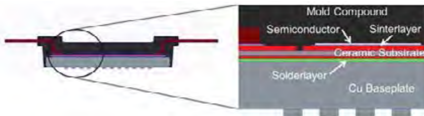
Figure 2: Thermal stack of the power module
