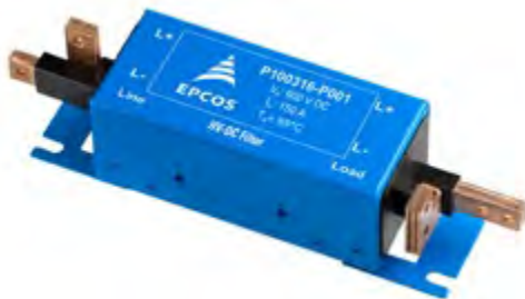
Figure 4: EPCOS high-voltage DC filters for automotive inverters. The connections of Version P001 are formed in such a way that they can be connected directly to the EPCOS DC-link capacitor. Apart from the space-saving design, they also offer electrical advantages such as low inductance and contact resistances.
