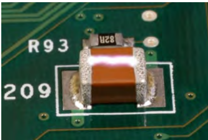
Figure 1: Surface arcing between MLCC terminations
