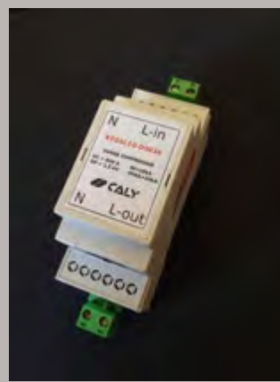
Figure 4: Presently available only as a DIN module CALY Technologies' hybrid SPD could soon be available as a much smaller form factor 3-pin module and the company is working closely with Raytheon UK's Semiconductors Business Unit in Glenrothes regarding the fabrication of the SPD's SiC-based Current Limiting Diode.
