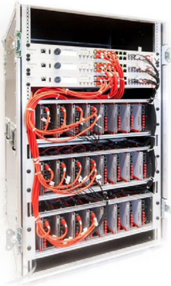
Figure 3: Modular multilevel converter prototype
