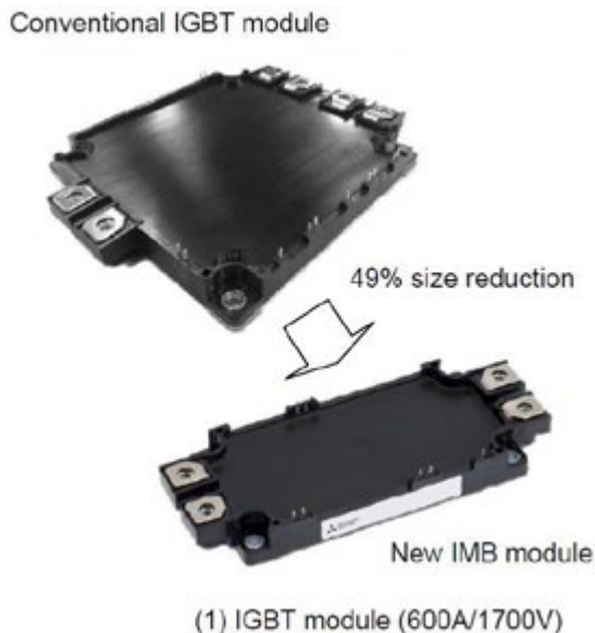
Figure 5: Example of the improved 1700V IGBT module by the new IMB
