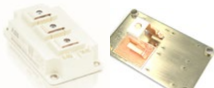
62Pak IGBT module (left), Spacers for homogenous solder thickness (right)
