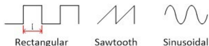
Figure 2: Possible pulse shapes at switch-on
