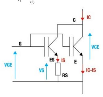
Figure 2: The basic concept of the current sense function
