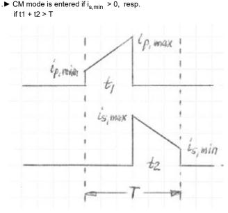
Fig. 5. Waveforms in CM
