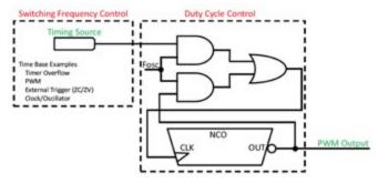
Figure 3: PWM implementation using CLC and NCO
