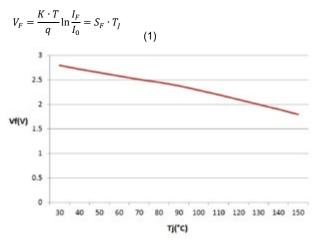
Figure 1: Dependency of voltage drop VF on the junction temperature Tj
