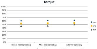
Relative thermal resistance by 2Nm mounting
