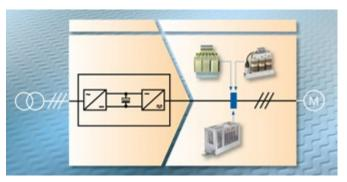
Moreover, the steep rising edge of the converter voltage excites parasitic oscillating circuits that consist of cable and motor capacitances as well as line inductances. Their transient characteristics overlay the converter voltage. On the motor side, this primarily results in momentary voltage overshoots which can far exceed the rated motor voltage (Fig. 1) and exert a load on the motor insulation due to partial discharges, which in turn can cause a motor to fail.
