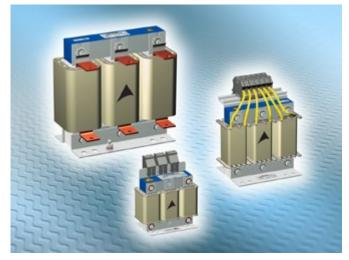
Figure 2: Motor chokes suppress voltage spikes The extensive range of EPCOS motor chokes covers a range of currents from 8 A to 1500 A. These prevent voltage spikes in the motor windings and thereby extend the service life of the motors.
