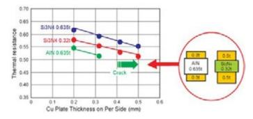
Figure 1d: Comparison of AMB substrates' thermal resistance 5
