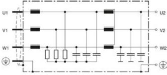
Figure 3: Circuit diagram of EPCOS SineFormer The SineFormer attenuates both symmetrical and asymmetrical interference. This eliminates the need for expensive shielded cables and protects the motor.
