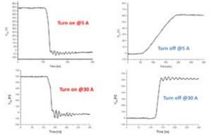
Figure 4: Turn on and turn off of the CoolSiC module within a DC/DC converter at 5 A and 30 A
