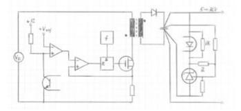
Fig. 2. FB converter with current mode control and galvanic isolation.
