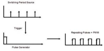
Figure 1: PWM construction
