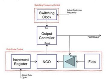
Figure 2: NCO-based principle of operation
