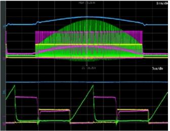
Figure 4: Inductor Voltage with Snubber Active (left) and Snubber Disabled (right) Legend: Magenta –inductor voltage; Green – inductor charging current; Yellow – Gate voltage for MOSFET; Blue – power line current Lower half of the picture is a zoom of the top portion at the position of vertical white lines
