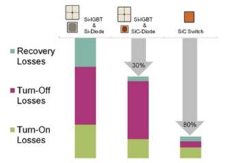
Figure 3: Evolution of loss reduction by the use of SiC power devices
