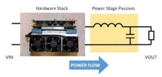
Figure 2: Synchronous buck with external inductor and capacitor
