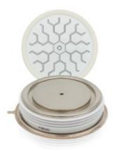
Melting systems, surface hardening or preheating – Induction heating applications are manifold. ABB's fast thyristors deliver the performance induction heating applications are asking for. ABB's family of fast switching thyristors are available with blocking voltages from 1,200 to 3,000 volt, average forward currents from 500 to 2,700 ampere and turn-off times from 8 to 100 microseconds. For more information please contact us or visit our website: www.abb.com/semiconductors
