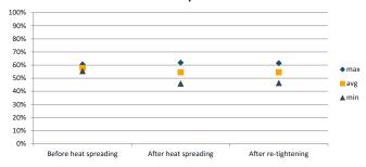
Figure 2: Rth measurement before and after heat treatment and retightening
