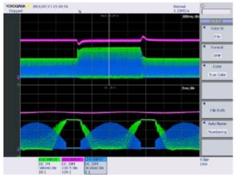
Figure 10: Scope snapshots depicting feedback reaction on a load boost from 60% to 100%
