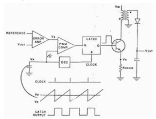
Fig. 1. Basic FB circuit with voltage mode control.
