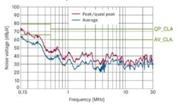
Figure 4: Noise voltage measurement on EPCOS SineFormer. Despite the unshielded cables, the permissible limits are observed.
