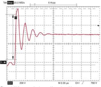
Figure 1: Voltage overshoot caused by motor cable
