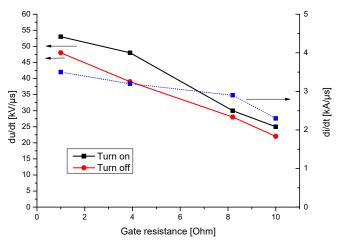
Figure 5: Controllability of the CoolSiC MOSFET via external gate resistors and the corresponding di/dt and du/dt levels
