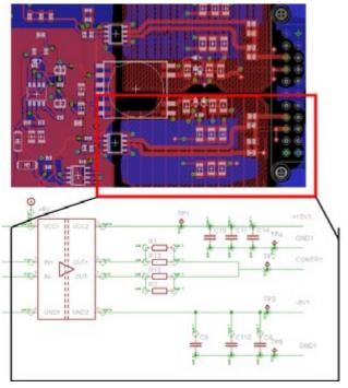
Figure 6: Example of a simple driver circuit for the CoolSiC MOSFET using Infineon's new compact driver 1EDI60H12AH
