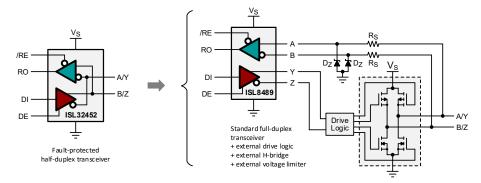
Figure 3: Integrated versus discrete over-voltage protection designs
