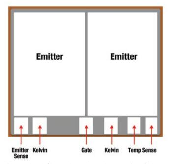
Figure 4: Layout of temperature and current sense pads on the top side of the IGBT
