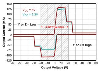
Figure 4: Driver output current limiting versus over-voltage
