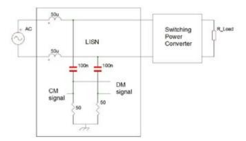
Figure 2: Conducted EMI testing with a LISN
