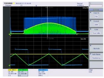
Figure 12: Scope snapshots depicting power line current along with inductor current and voltage
