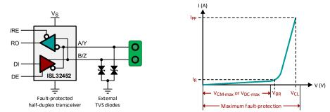
Figure 5: TVS V-I characteristic in comparison to V<sub>CM</sub>-max and V<sub>DC-max</sub>
