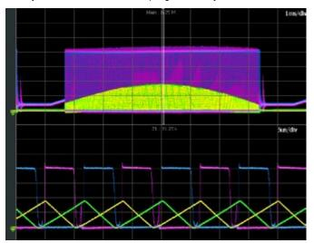
Figure 2: General Waveforms of Two-phase MCU-controlled PFC Converter
