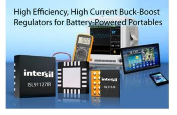
ing system power or powering the peripherals in battery-operated devices. They offer the industry's lowest quiescent current of  $30\mu A$  for superior light load efficiency.
