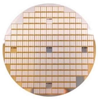
Figure 5: Wafer with bare-Die IGBTs as presented at PCIM Europe, 2016
