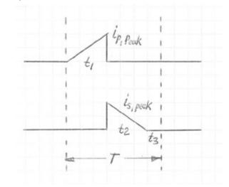
Fig. 3. Waveforms and definitions for DCM.
