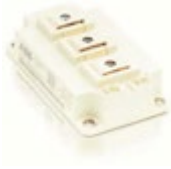
Figure 1: The 62Pak (standard footprint of 62mm x 106.4mm) module using the third generation ABB SPT ++ chipset for high temperature module operation (nominal conditions: V_{DC}=900\text{V} , I_C=300\text{A} or I_C=200\text{A} , V_{GE} = \pm 15\text{V} , L_s = 60\text{ nH} and R_{Gon} = R_{Goff} = 2.2\text{ W} or R_{Gon} = R_{Goff} = 2.7\text{ W} for I_C=150\text{A} version, respectively).
