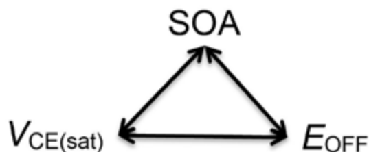
Figure 2: Fundamental trade-off for IGBT characteristics
