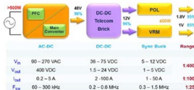
Figure 2: Plug to Processor power train with operating parameter ranges in each stage
