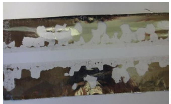
Figure 4: Demetallized electrodes by corona arcing in the air gap between the films
