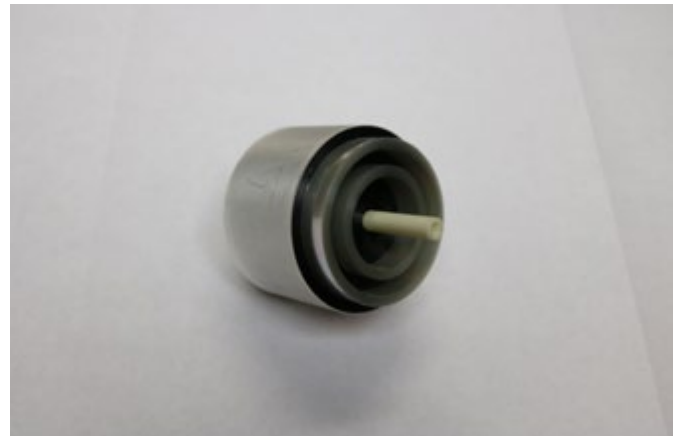
Figure 5: Triple concentric winding of a true coaxial capacitor
