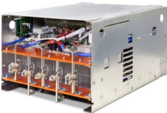
Figure 3b: Air cooled cell showing rectifier modules (black) in the center and 62mm modules (white) on the right and left.
