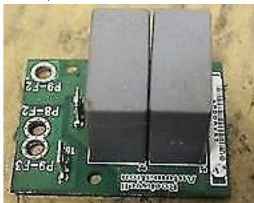
Figure 3: Snubber circuit with reversed current flow in box capacitors
