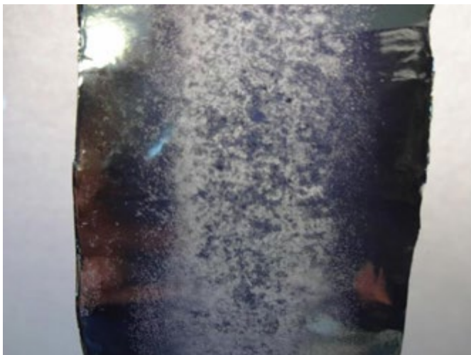
Figure 5: Electrode corrosion due to the presence of humidity
