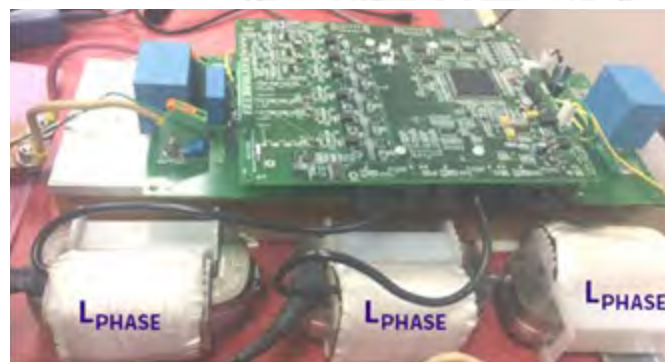
Figure 4: High-level technical specifications, 2L six-switch AFE power stage circuit topology, and realized 20kW AFE hardware prototype based on 2x C3M0065100K per switch position.
