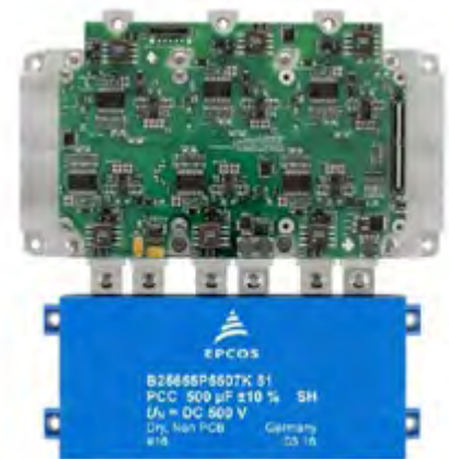
Figure 3: The busbar of the EPCOS PCCs has six large terminals and ensures that the ESL and ESR are minimized.
