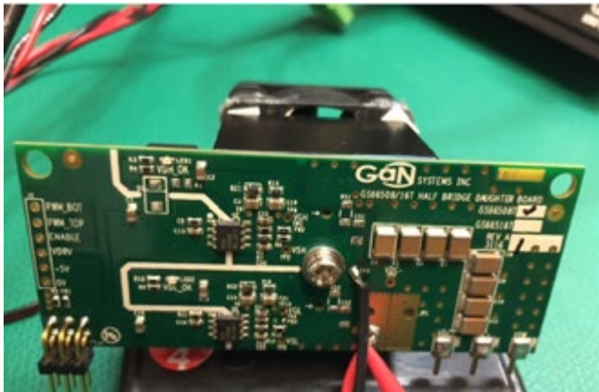
Figure 10: GS66508T Thermal Resistance Setup
