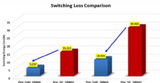
Figure 8: 400 V / 15 A GS66508T and C3M0065090J Switching Loss Comparison
