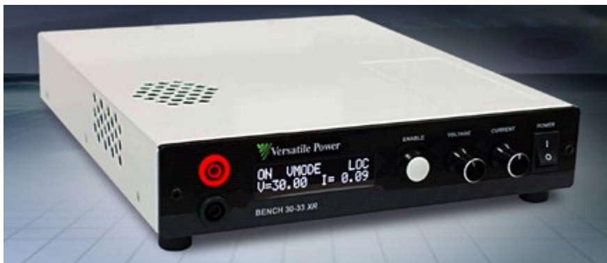
Figure 3: The Versatile Power Bench XR power supply uses patent pending digital remote sense to eliminate wires
