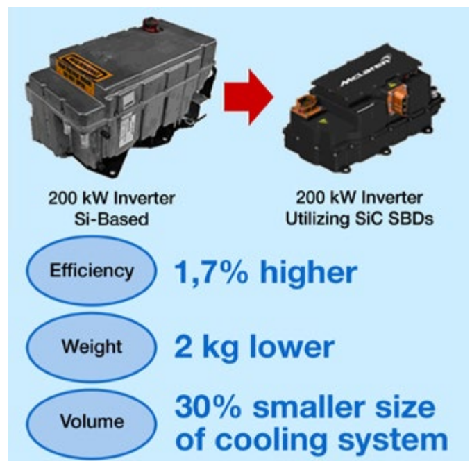
Figure 4: Improvement of performance and size reduction in power train inverter with SiC SBD technology for Formula-E racing car
