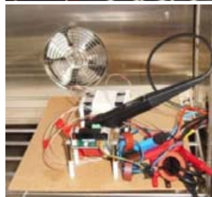
Figure 4: Calorimeter set-up for analysis of the power losses in the output choke with sensors and terminals
