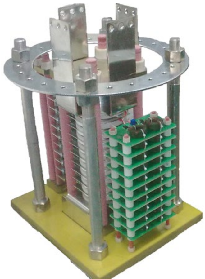
Figure 7: Experimental thyristor switch for commutation of current pulse with 250 kA amplitude.
