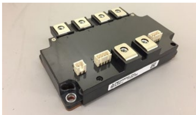
Figure 8: Advanced 800A/1200V full SiC Dual module FMF800DX2-24A
