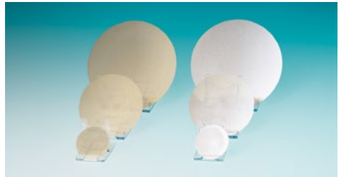
Figure 2: SiC Wafer with different diameters (2, 4 & 6 inch) after splitting using identical process parameters for COLD SPLIT.
