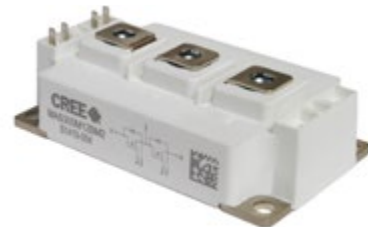
Wolfspeed Figure 2: First All-SiC module to achieve this new reliability benchmark
