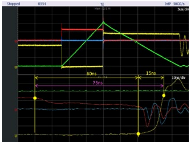
Figure 1: Boost Switching of SJ IXFH50N85X in a Typical Application Legend: Yellow – Inductor/Drain Voltage; Green – inductor current; Red – gate voltage; Note: The bottom of the scope snapshot is a zoom of the top portion of the area between two white lines.
