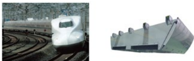
Figure 13: First All-SiC propulsion inverter in Shinkansen Bullet Train
