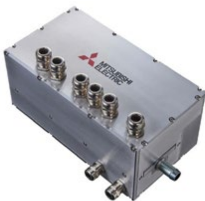
Figure 18: Ultra-compact inverter with 86kVA/dm 3 for HEV
