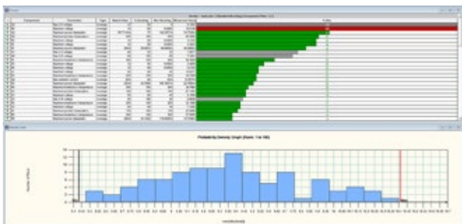
Figure 3: Example showing stress and component tolerances (Monte Carlo Analysis) to improve overall reliability
