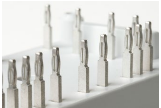
Figure 4: Press-fit pins for solder less mounting
