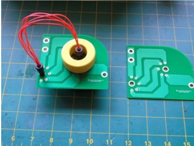
Figure 2: JIG, core can be insert / removed before / after measurement by plug the center pole
