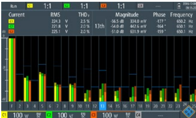
Figure 8: Harmonics analysis of a three-phase 100 V signal. The blue lines show the current limit value in line with EN 50160. The 13 th harmonic and its characteristics are highlighted; the highlighted levels for the three channels lie between -56.5 dB and -51.0 dB; source: Rohde & Schwarz
