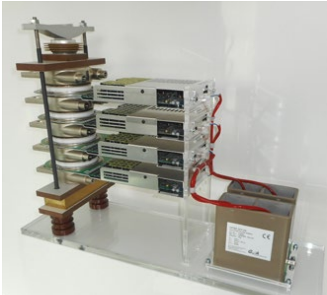
Figure 2: The new GPSS is the perfect insulating supply unit for IGBT and IGBT stacks.
