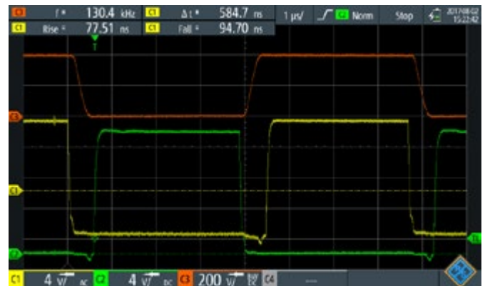
Figure 1: Measuring the gate source (C1, C2) and output voltage (C3) of a resonant converter; source: Rohde & Schwarz
