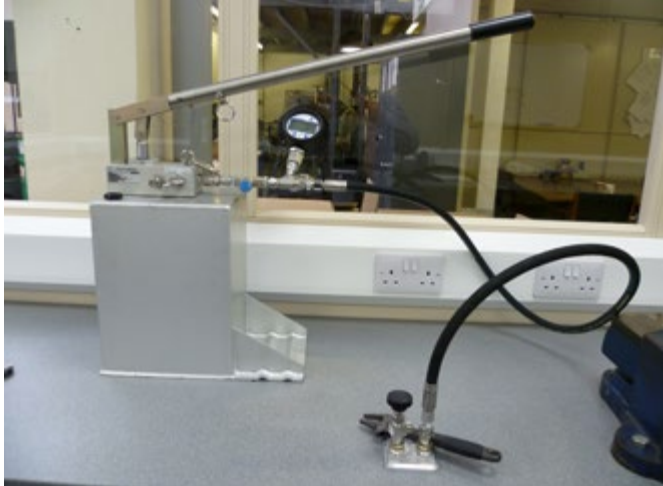
Figure 3: Withstand proof pressures in the region of 10bar
