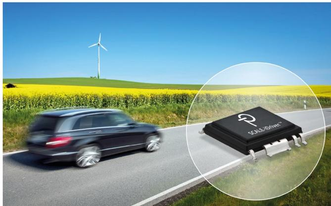
A and +/-8 A respectively. The SID1182KQ has the highest output current of any isolated gate driver available and is capable of driving a 600 A /1200 V and 820 A /750 V switch.
