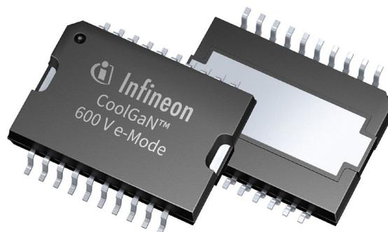
The performance of CoolGaN is beyond other GaN products in the market. At 100 ppm (parts per million), its predicted lifetime is about 55 years, exceeding the expected lifespan by 40 years. CoolGaN enables for example doubled output power in a given energy storage slot size, freeing up space and realizing higher efficiency at the same time.
