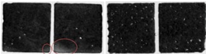
Figure 4: The image on the left is a standard preform showing solder joint delamination after 600 cycles. The image on the right is a solder joint formed with a reinforced solder that shows no delamination after 800 cycles.
