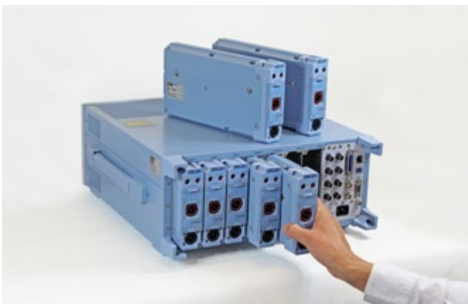
Figure 4: The WT5000 has seven built-in slots for user-swappable power input modules and mainframe options that enable users to expand or reconfigure the WT5000 as their requirements change.
