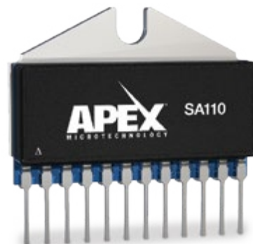
12-PIN, POWER SIP, STYLE DP WITH HEAT TAB
