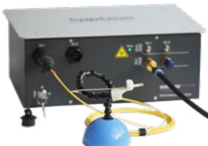
Figure 1: Electro-optic probe and associated optoelectronic converter.
