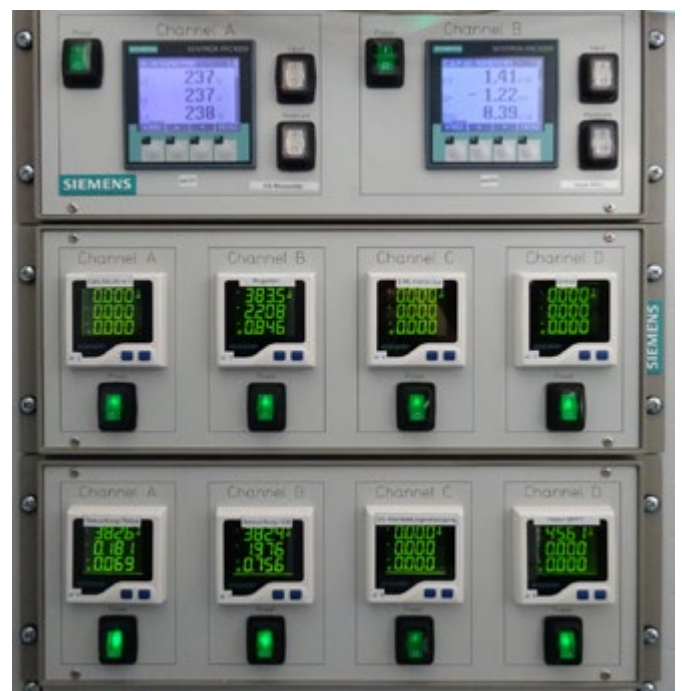
Figure 2: Mixed AC/DC-power monitoring system
