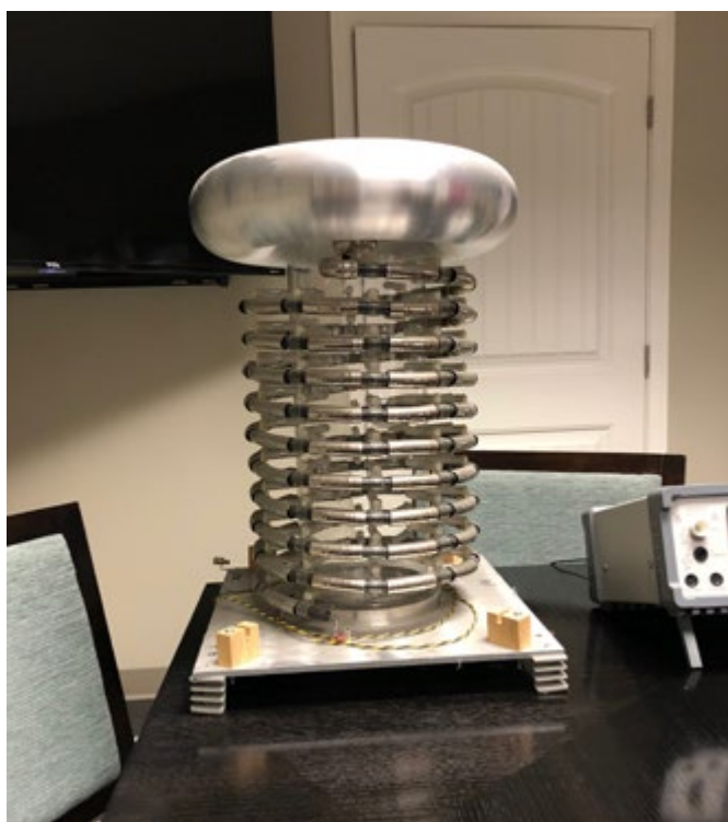
Figure 2: 100:1 voltage divider network built in compliance with the NIST standard.
