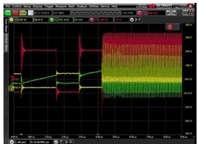
Figure 1: Example unexpected ringing seen at the double pulse test
