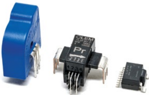
Figure 2: Evolution of the current sensor's size over the decades
