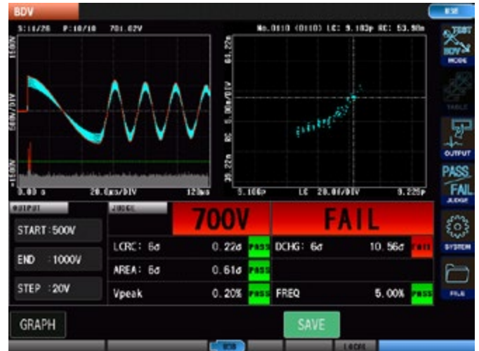
Figure 4: The ST4030A's BDV function
