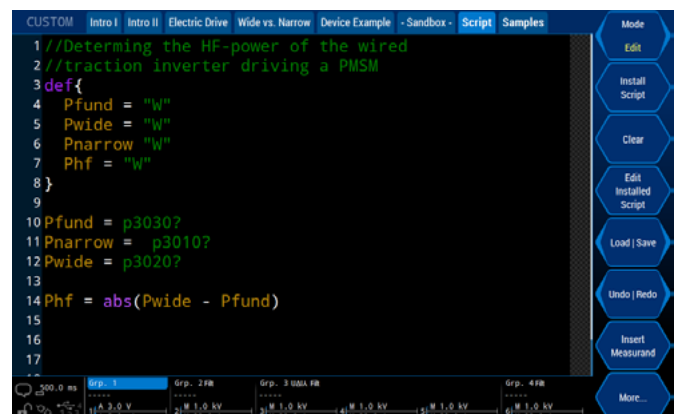
Figure 5: LMG671 script editor for calculating high-frequency power losses at the converter output
