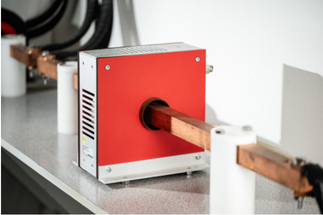
Figure 2: Danisense has its own ISO/IEC 17025-accredited calibration laboratory and offers brand agnostic calibration services for current transducers
