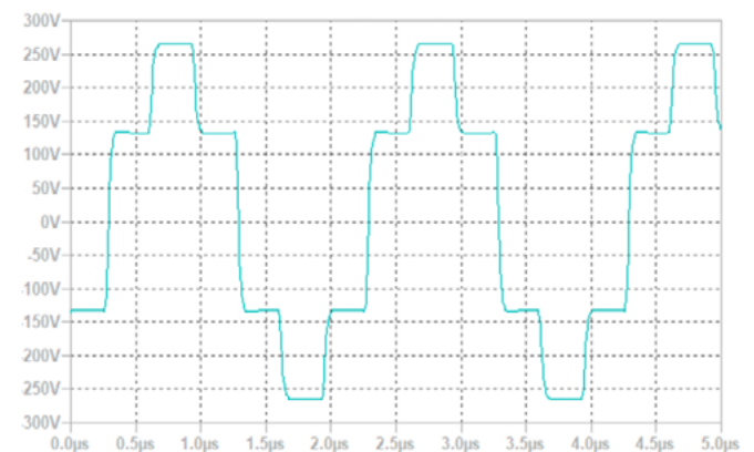
Figure 8: Primary phase-element voltage – the voltage between the output of the transistor bridge and the primary star point.
