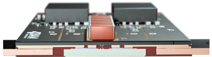
Figure 4: Cross section render of the GT1 Power Module.
