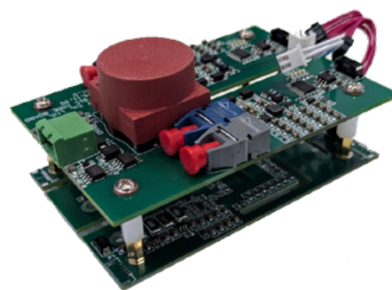
Figure 2: Silicon Carbide (SiC) Core Driver Board
