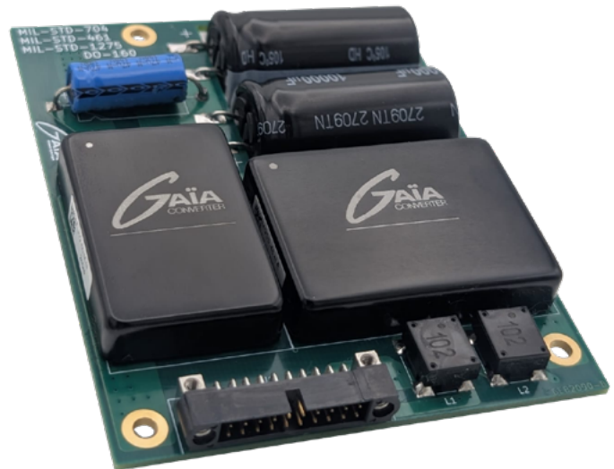
Figure 1: This 40 W power supply complies with Mil-STD-704, Mil-STD-461, Mil-STD-1275, and DO 160 standards thanks to its FLHG60, the latest integrated input front-end from GAIA Converter.
